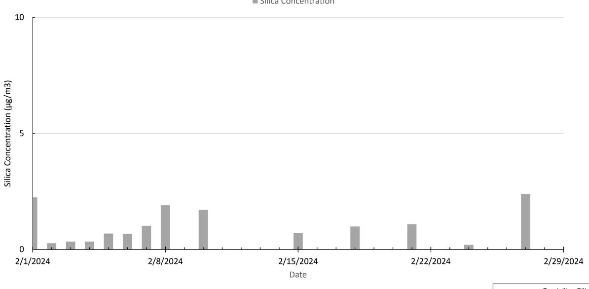
Crystalline Silica – Quartz 24-hour FRM sample North Station
