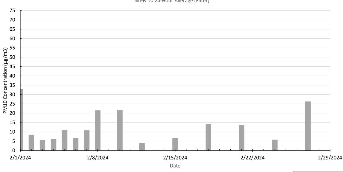
10-micron Particulate Matter 24-hour FRM sample North Station
