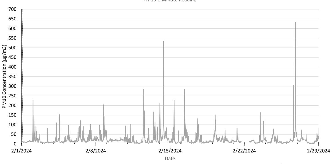
10-micron Particulate Matter 1-Minute FEM Data Fenceline Station
